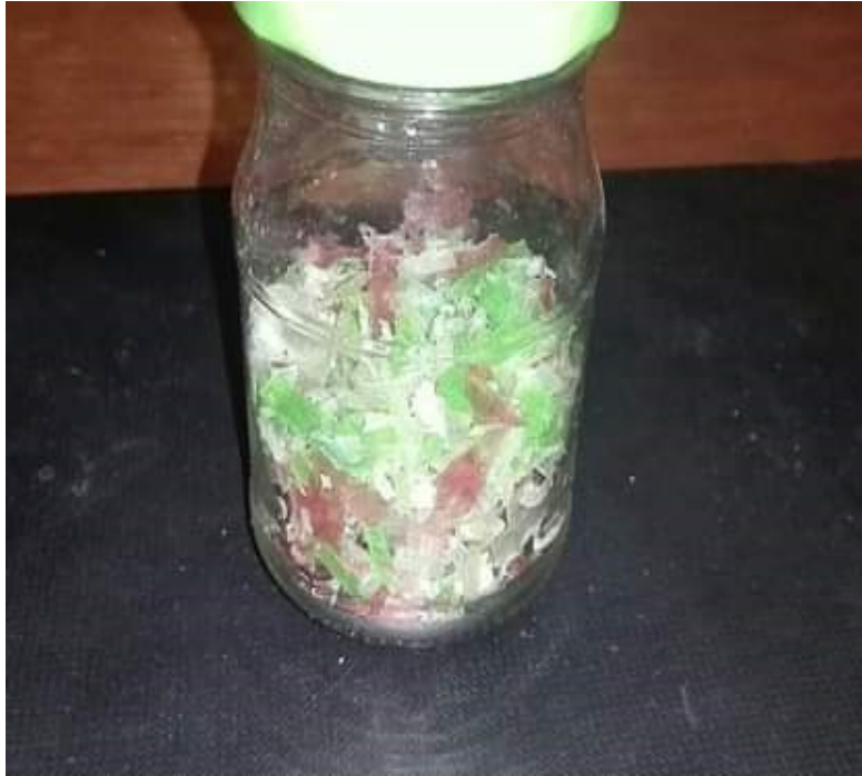
Figure 30. Shreds of hard bioplastic to be used in moulding process for the creation of hard type kitchenware like spoons and plates etc.
