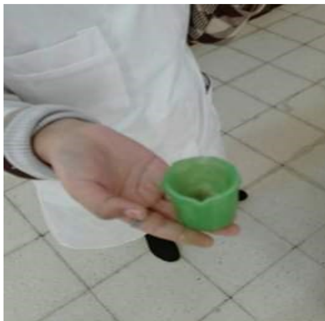
Figure22. Example of moulding a mass of bio-plastic into a beaker shape, see also Results and Discussion chapter.
