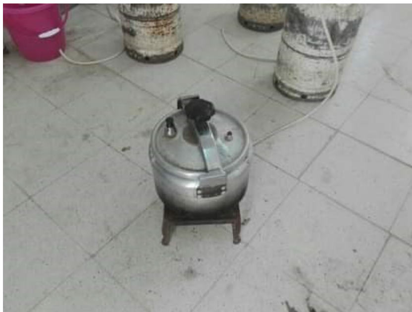
Figure 24. Pressure cook used to sterilize the culture media
