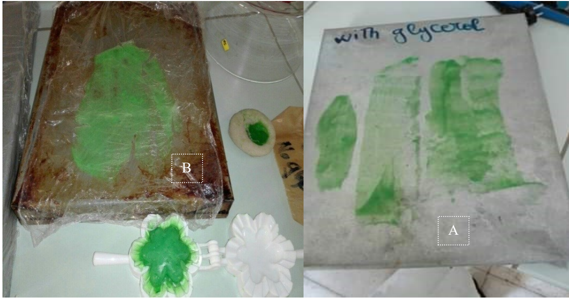
Figure 31. Flexible bioplastic coloured green; in sheet form [A] thin, [B] thicker and flower shaped blob [C] using a press mould.
