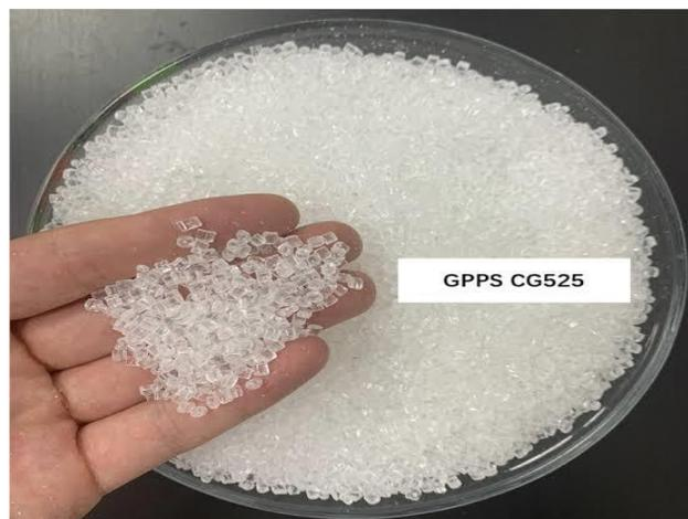
**Figure 9:** Polystyrène cristal.
