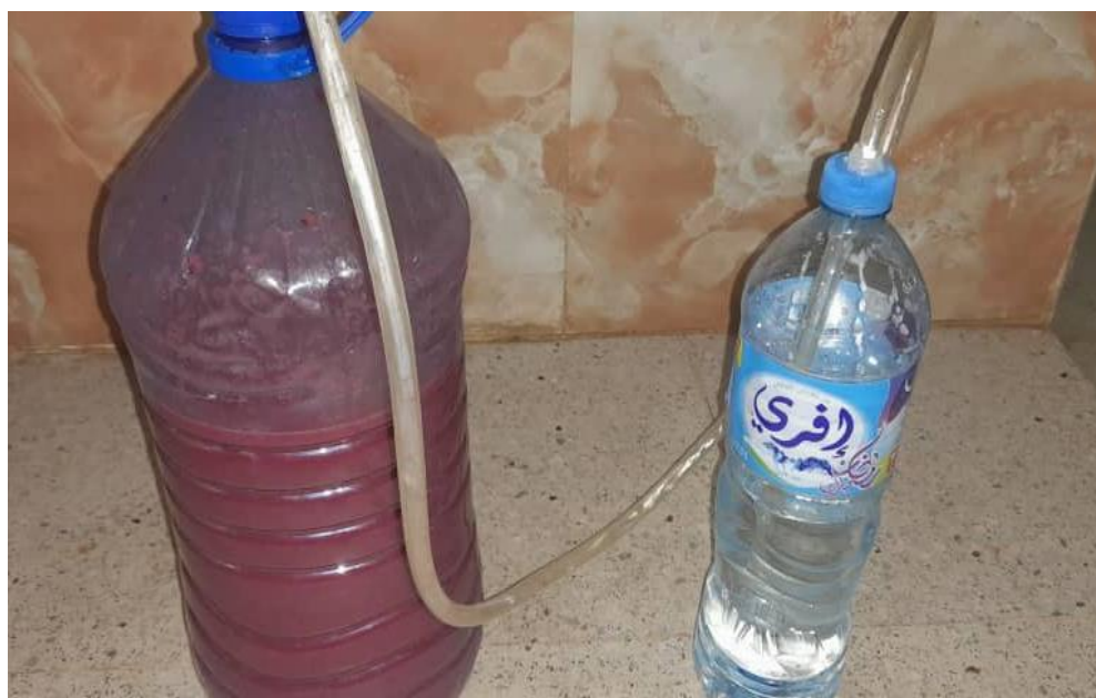
Figure 9: Fermentation of fruits and vegetables wastes broth in a sealed plastic jug.
