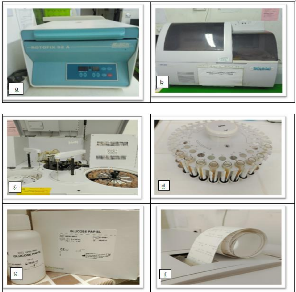
Figure 26: Materials used to Calculate blood sugar level ( a. Centrifuge , b. The Biolisautomaton, c. Samples in the automaton, d. Serum pipetting, e. The PAPSL glucose reagent, f. Exit result).
