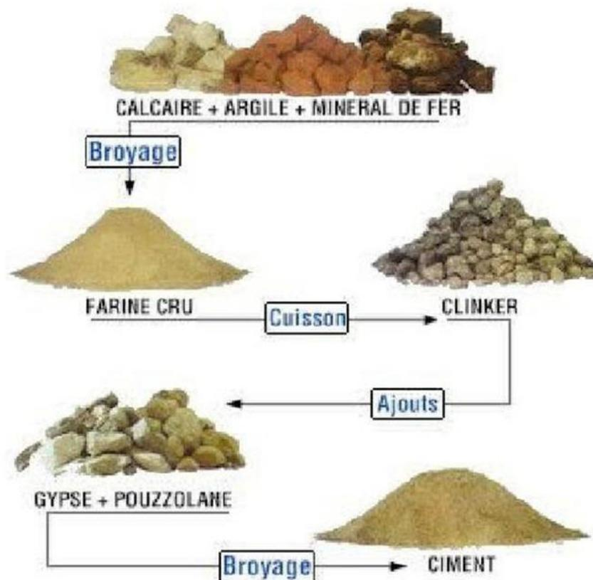
Figure 2.15 Processus de fabrication de ciment [61]
