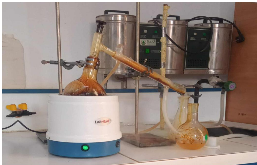
Figure II.2: Montage de hydrodistillation de juniperus
