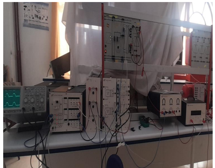
Figure (III.28) : Montage simple alternance charge inductive, (a) théorique, (b) simulation, (c) pratique.
