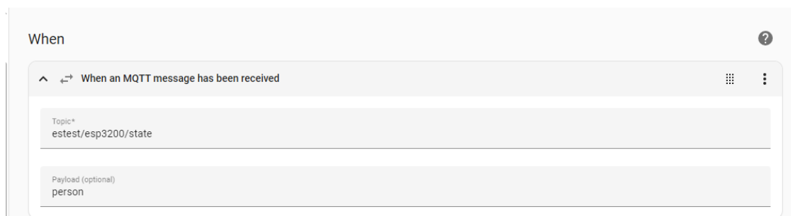
Figure 4.31: Conditional check for MQTT payload containing "person".
