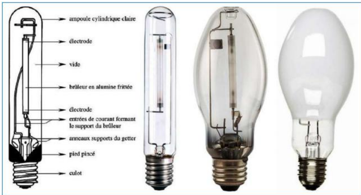
Figure 2.9. Structure standard des lampes SHP [76].
