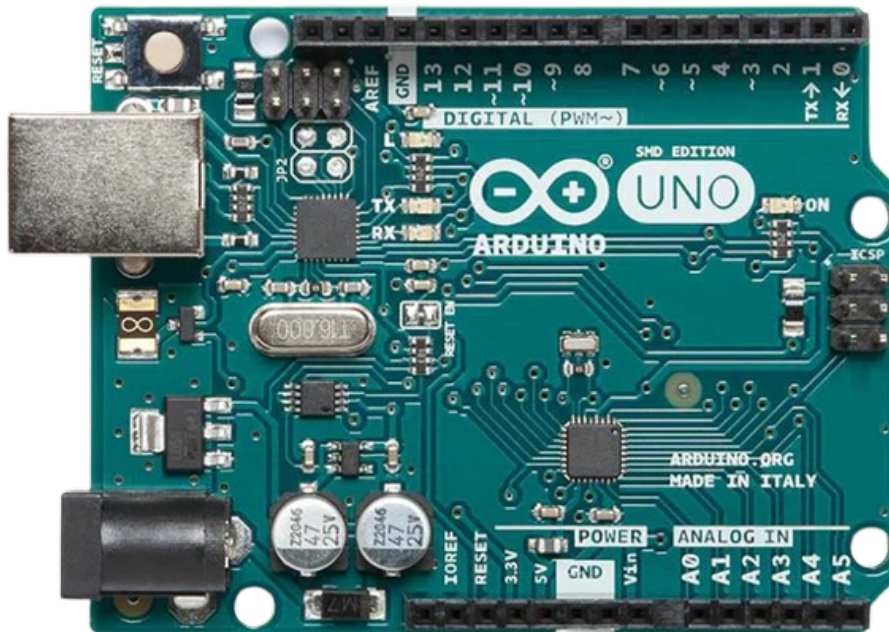
FIGURE 2.5 – Arduino Uno Board
