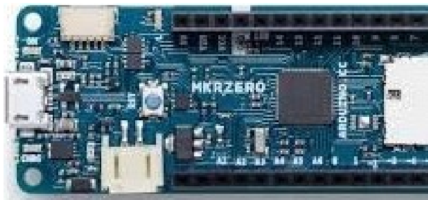
FIGURE 2.11 – Arduino MKR Zero Board
