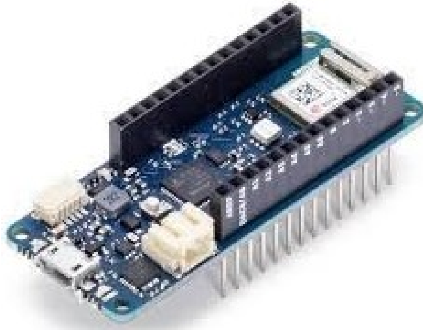
FIGURE 2.12 – Arduino MKR WiFi 1010 Board
