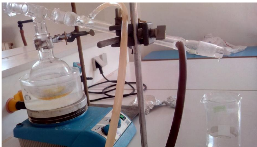
Figure B-1-3: Montage de distillation.
