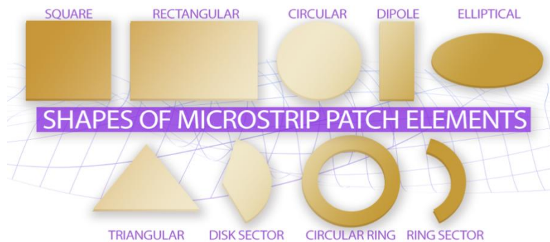
Figure II.17: Different patch shapes [22].
