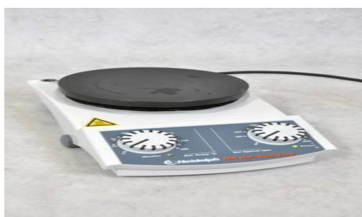
Figure B-1-1: plaque chauffante de type HEIDOLPH.
