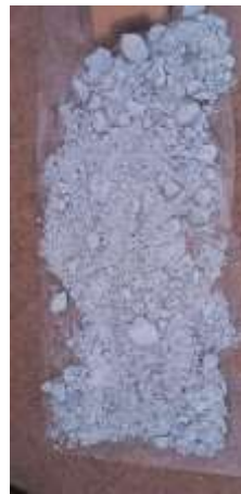
Figure III-8 : Drying of Carbide Lime Powder Under Sunlight
