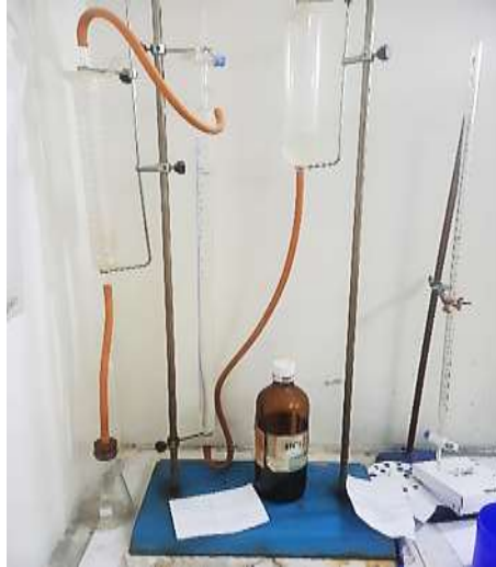
Figure II-10: Apparatus Setup for Determination of Carbonate Content by Calcimetric Method
