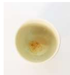
Crucible after furnace calcination
