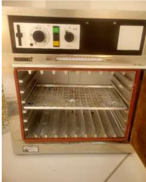
Figure II-1: Memmert Drying Oven used during Humidity Test
