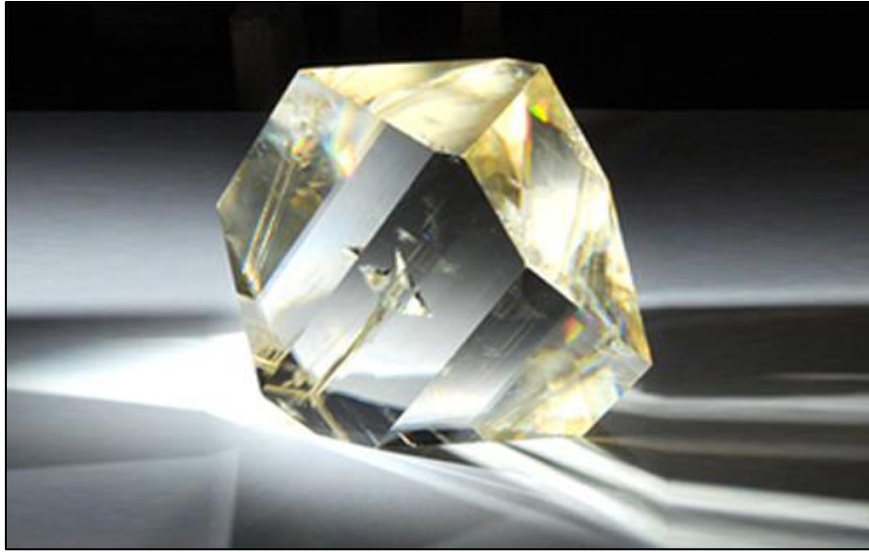
Figure I.6: Bêta-baryta borat (BBO) crystal (38).
