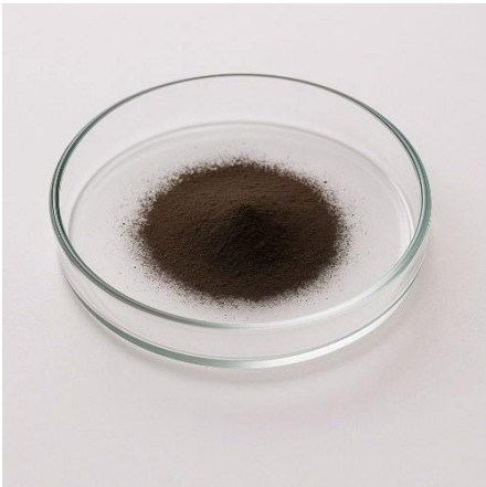
Figure 26. Biosynthesized Copper Nanoparticles (CuNPs) Recovered in Petri Dish After Purification and Drying
