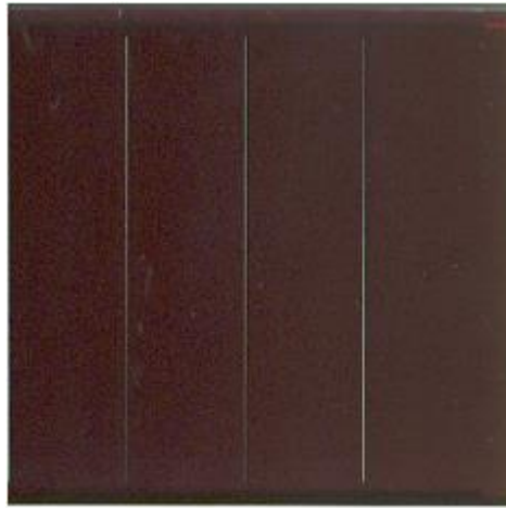
Figure (1.13) : Cellule photovoltaïque amorphe
