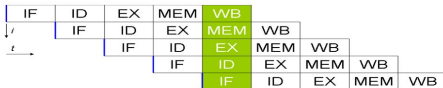
Figure 3.33: a canonical five-stage pipelined processor. in the best case scenario, it takes one clock cycle to complete one instruction and thus the processor can issue scalar performance ( ipc = 1 ).
