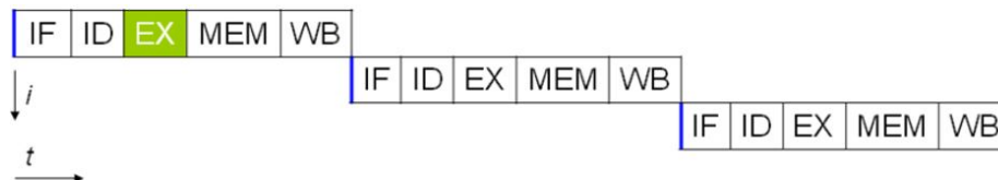
Figure 3.32: A canonical processor without pipeline. It takes five clock cycles to complete one instruction and thus the processor can issue subscalar performance ( IPC = 0.2 ).
