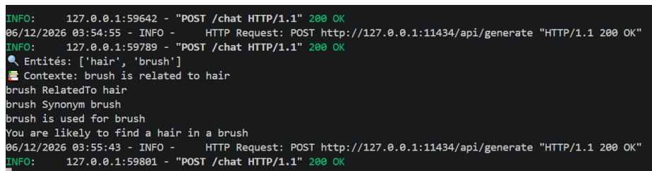
Figure 18 – Backend logs: extracted entities ['hair', 'brush'] and retrieved ConceptNet relations. Source: Author’s own screenshot.
