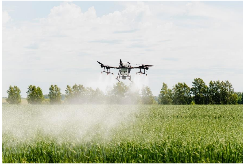
Figure 2.5. A modern agricultural drone with a tank and spray arms. Drones are modular: the camera and the tools can be changed for each task, which shows how flexible they are [41].
