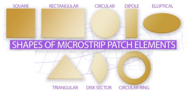
Figure II.2: The most common shapes of patch antennas [5].
