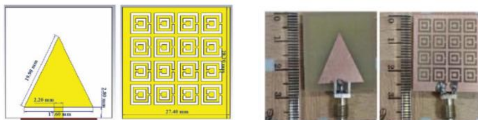
Figure II.14: Geometry and Fabricated triangular patch antenna with CSSR on the ground plane [23].
