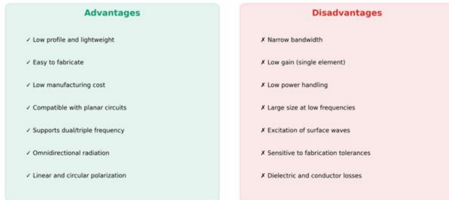
Figure 1.9 — Summary of advantages and disadvantages of microstrip patch antennas.
