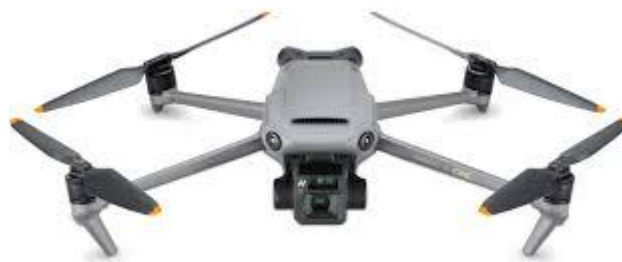
Figure IV.1: DJI Mavic 3 Cine UAV used for acoustic signal acquisition.
