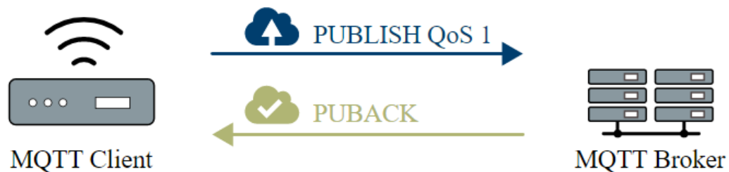
Figure 22: MQTT Quality of Service level 1: delivery at least once
