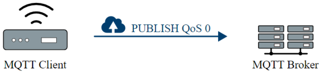
Figure 21: MQTT Quality of Service level 0: delivery at most once
