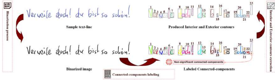
Figure 4.4: Preprocessing of an example handwritten text line taken from CVL [31] database (from [4]).
