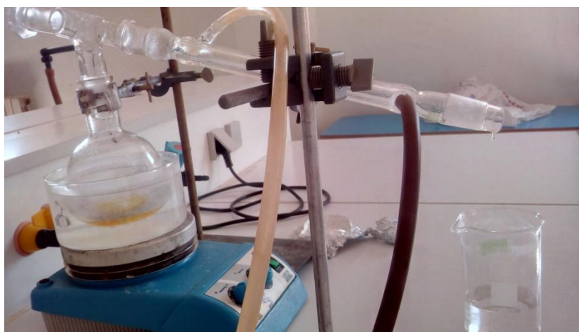
Figure B.1.3: Montage de distillation.
