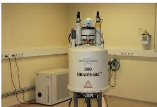
Figure B.1.8: Appareil RMN de type BRUCKER AM (300MHz).
