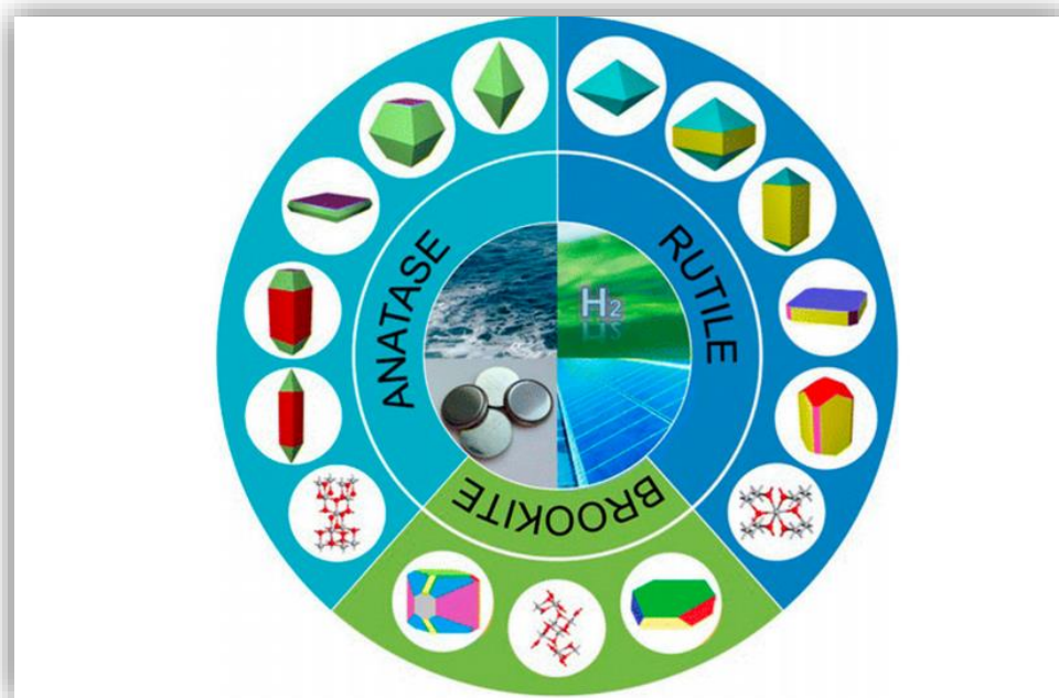
Fig II.11 Summary of main shapes and applications (i.e., lithium-ion batteries, photocatalytic hydrogen evolution, photodegradation, and solar cells) of anatase, rutile, and brookite \text{TiO}_2 crystals with their surfaces consisting of different Facets
