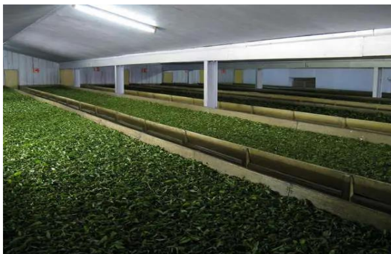
Figure 10 : Withering process to reduce leaf moisture content (Planted Well; 2022).
