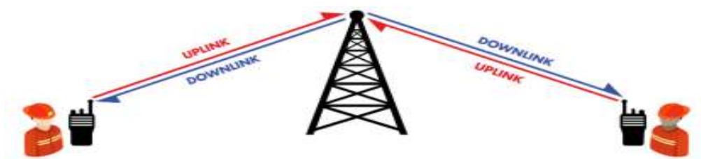
Figure 2.3: Uplink and Downlink.
