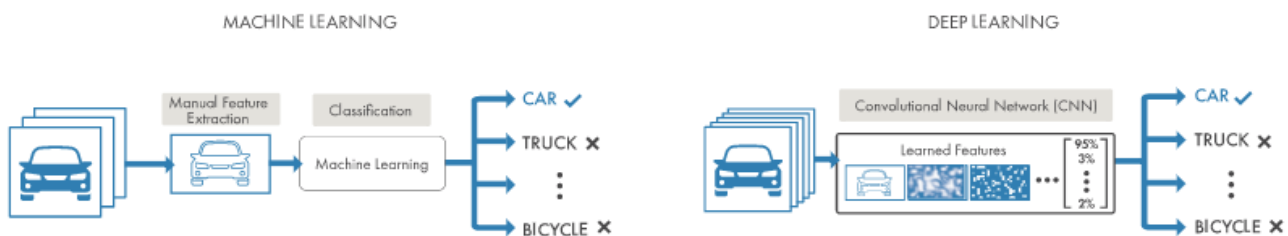
Figure 11 :Comparison between a machine learning approach (left) and a Deep Learning approach (right) in an example of vehicle classification[9]
