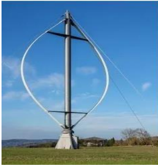
Figure I.3: Darrieus Vertical Axis Wind Turbine. [10]
