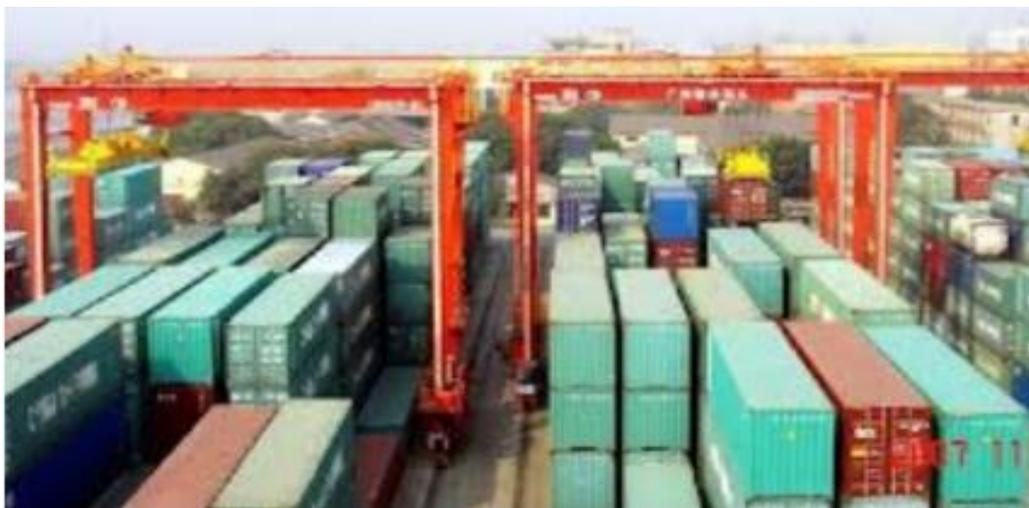
Figure7: Rail-Mounted Gantry Crane (RMGC). [6]
